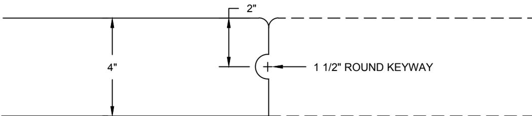
**TEMP. END OF WORK NOT ENDING AT AN EXPANSION JOINT**
