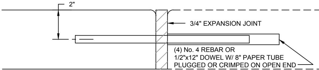
**END OF SIDEWALK RUN OR AT EXPANSION JOINT, APPROXIMATELY 100' INTERVALS**
